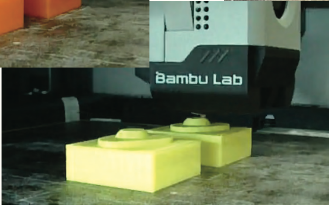
3D printing using Bambu Lab X1 Carbon 0.4 nozzle
